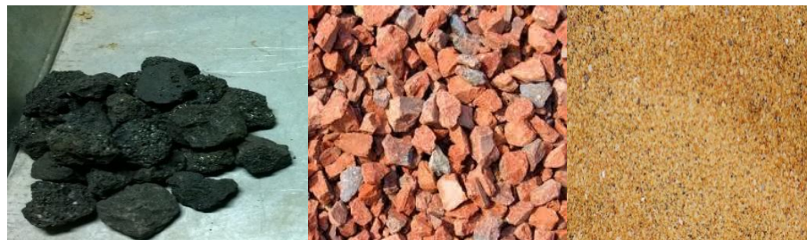
Figure 1: Different Types of Aggregates (Left-Mixed Slag, Middle- Brick Chips, Right-Sylhet Sand)
