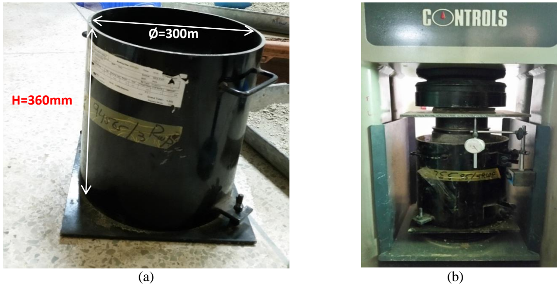
Figure 1: Steel moulds: (a) Dimensions (b) Mould loaded in Compression Testing Machine
