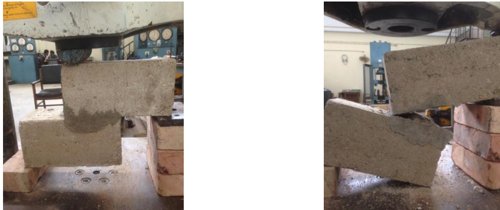
Figure 7. Z-Shaped Specimen (Flexure Bond Strength)
