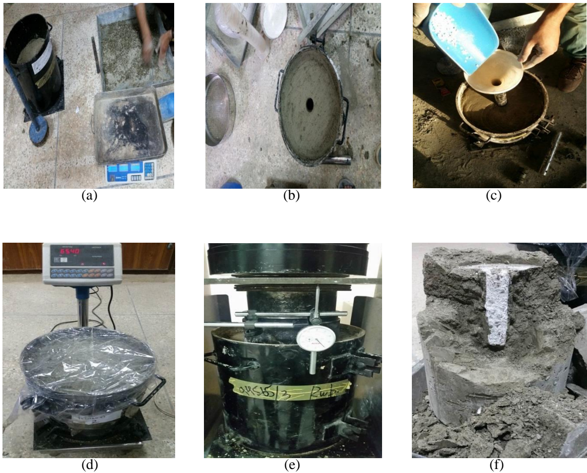
Figure 3: (a) Mixing and compacting soil (b) Borehole for column (c) Pouring column material (d) Model wrapped for curing (e) Model testing (f) Failure pattern of composite model
